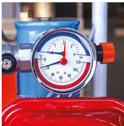
Manometro e termometro. Pressure gauge and thermometer.
